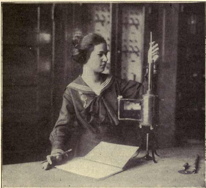
TAKING THE TEMPERATURE OF STEAM OVER BOILING WATER TO DETERMINE THE BOILING POINT.
